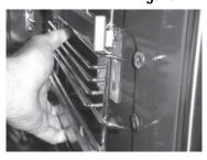
To remove the oven rack support for a self-clean cycle, support and lift front bottom of rack support to release front tabs. Then, rotate rack support up and out to release rear tabs. If the rack supports are not removed, the self-clean cycle won't start. Figure 15
